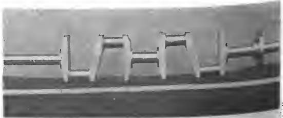
Balanced Four-Cylinder Crankshaft of Alloy Steel.
